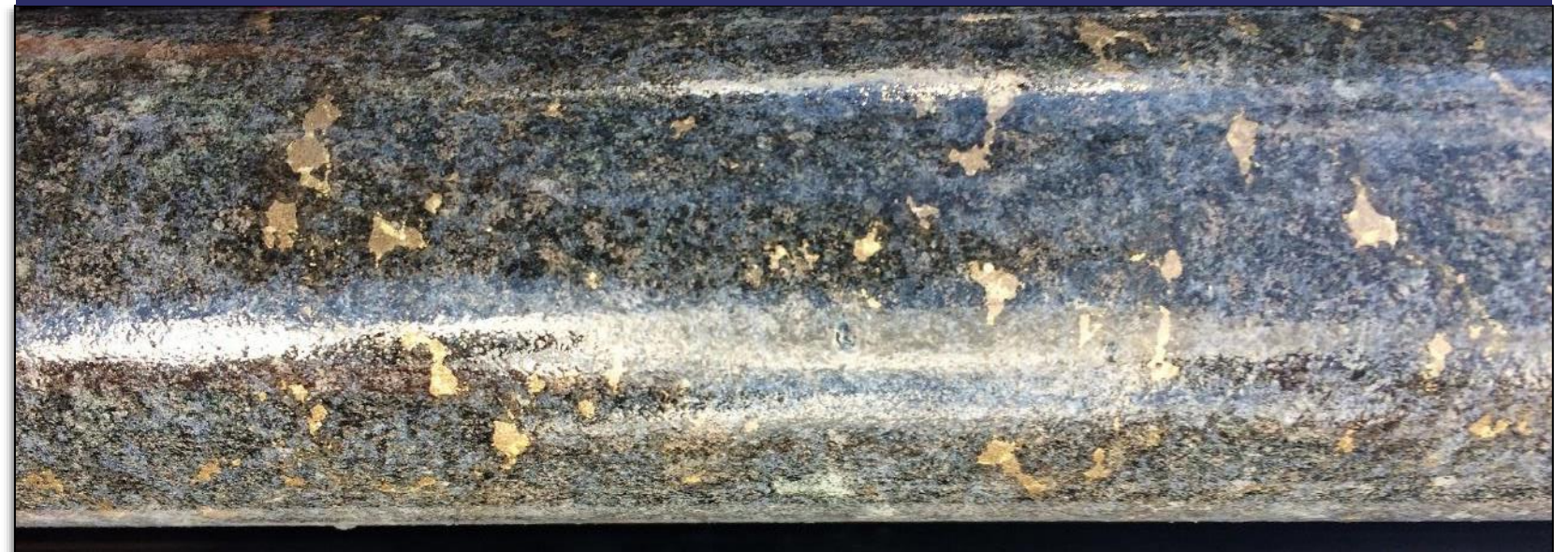
SFRD0711 @ 312m. Sulphides in Gabbronorite, NQ2 Core
