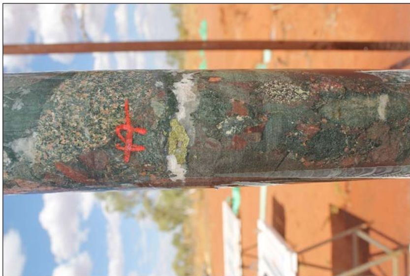
Photo 1. Polymictic breccia with vein hosted blebby chalcopyrite in EPT2276 at Aria
