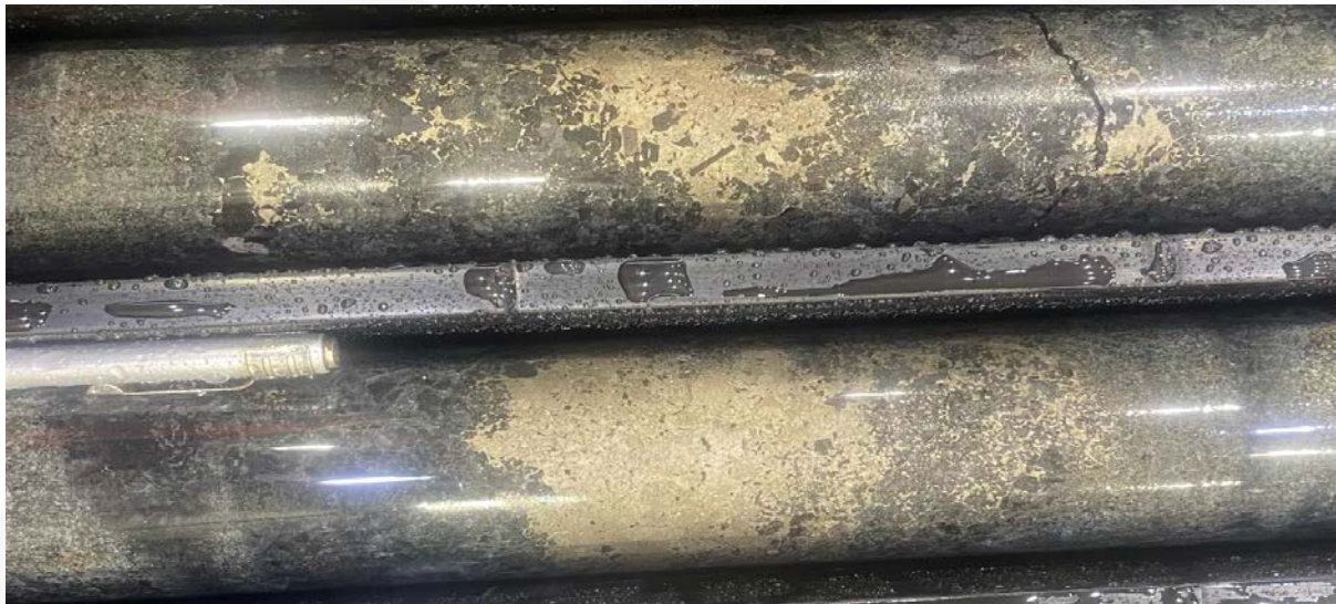
Figure 4: Semi massive three-phase sulphides in cumulate gabbro-norite at 576.8m in 21AFDD105 (core size is NQ2; 50.6mm diameter)
