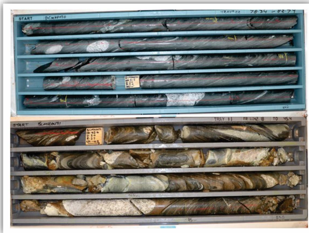
Figure 4: Drill core from BCMH0070 and BCMH0071 showing metamorphosed conglomerate with granitic cobbles in sheared mafic matrix
