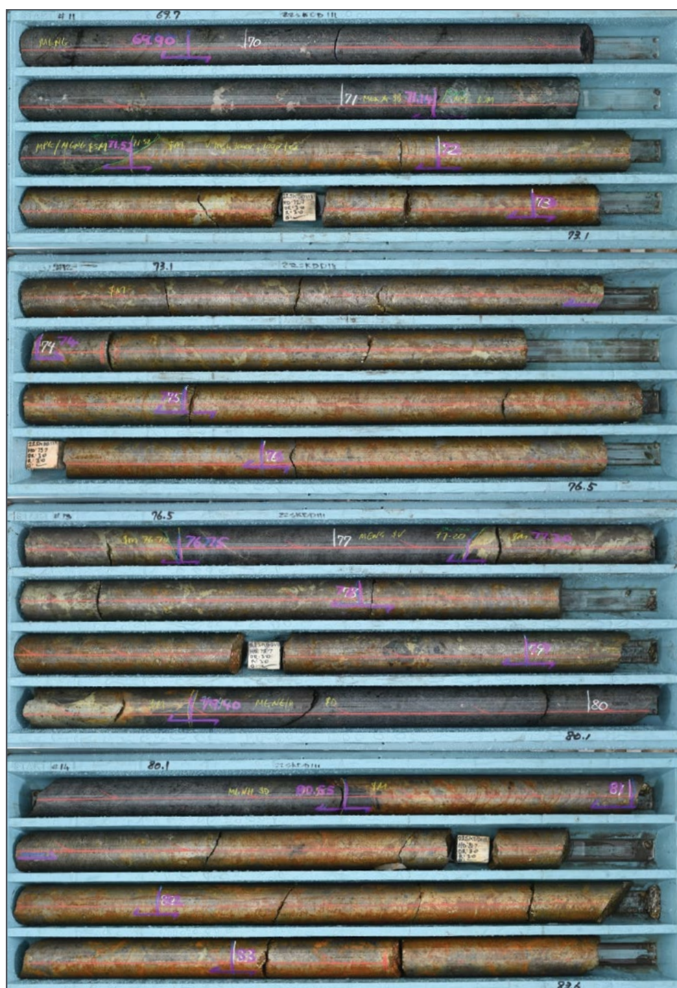
Figure 10: 22SKDD111 Ni-Cu-Co mineralisation in drill core
