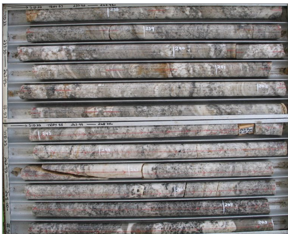
Figure 21: SID022 spodumene bearing pegmatite at South Ironcap Prospect
