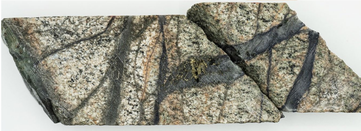
Figure 2: HQ3 core from CPW0002D at 530.65 m depth. Cross-cutting quartz-sulphide veins carry chalcopyrite, pyrite and molybdenite sulphides. The granitic host rock has been altered by an early clay alteration which has been overprinted by K-feldspar (as vein selvage) and later sericite. Visually estimated sulphide abundances: 2.25% pyrite, 0.8% chalcopyrite and 0.15% molybdenite. HQ3 core is 63.5 mm width.
