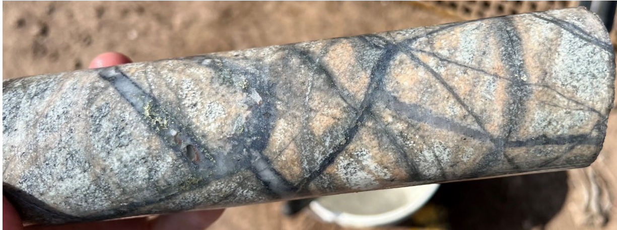
Figure 6: Whole HQ3 core from 710.00 m in CPW0002DD. Medium grained intrusive rock cut by multi-stage (stockwork) quartz-sulphide veins. This sample illustrates strong fine grained molybdenite mineralisation in banded quartz veins and distinct K-feldspar selvages. Visually estimated sulphide abundances: 4% pyrite, 1.25% chalcopyrite, 0.5% molybdenite. HQ core is 63.5 mm width.
