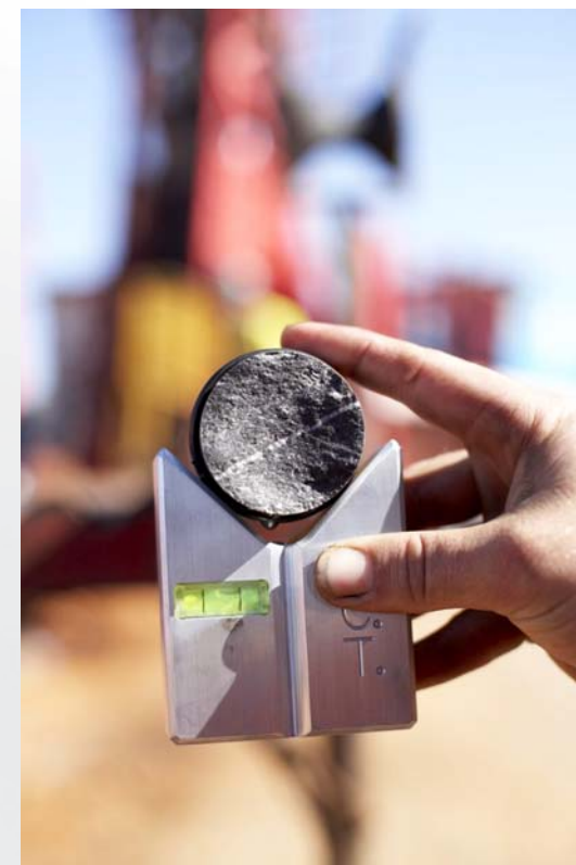
Drill core sample being oriented
