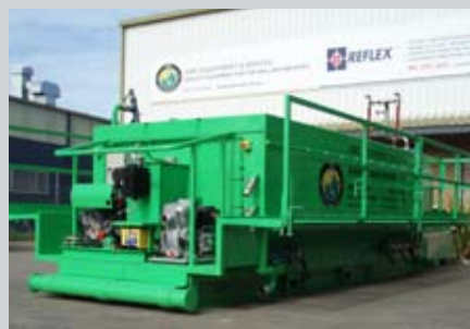
Surface Solids Control Unit
