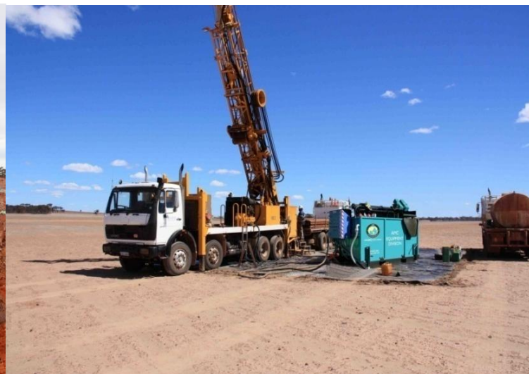
No sumps – fully enclosed system
