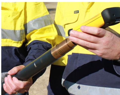
The Reflex Gyro undergoing testing in the field
