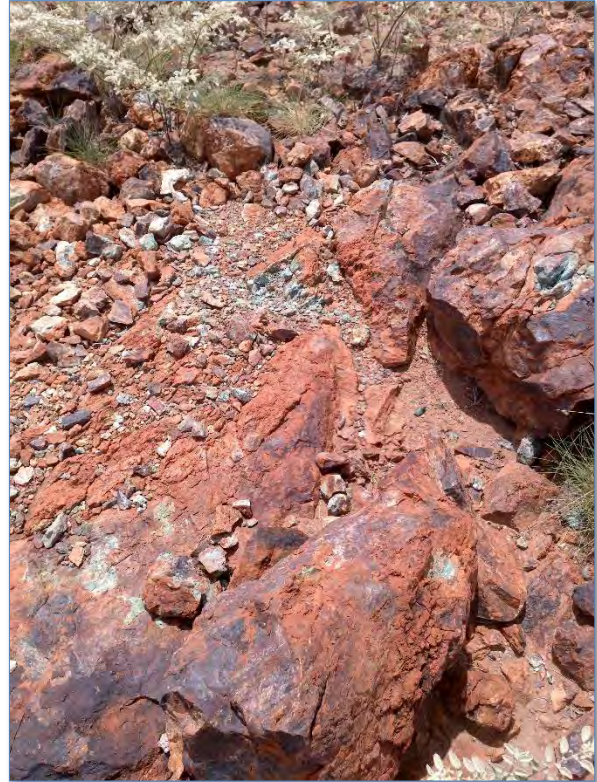
Photo 2: Hillside, vughy iron box worked silica rich rock with secondary copper minerals
