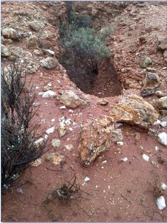
Photo 14: Victor Bore – carbonate altered quartz stock worked vein
