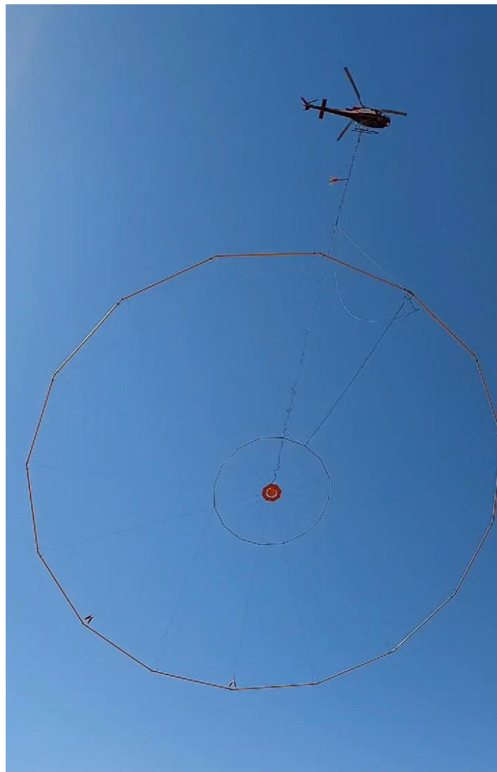
Figure 4: UTS Geophysics' Helicopter VTEM survey equipment
