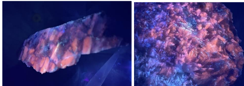
Figure 5. Woody (Tambourah South) rock chip samples under UV light showing spodumene as pink.
