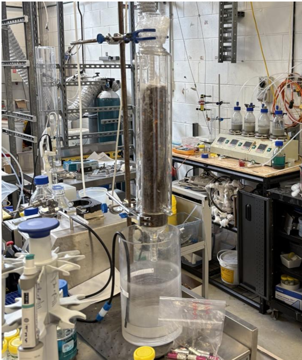
Figure 4: Orivium laboratory scale testing facility demonstrating metal extraction
