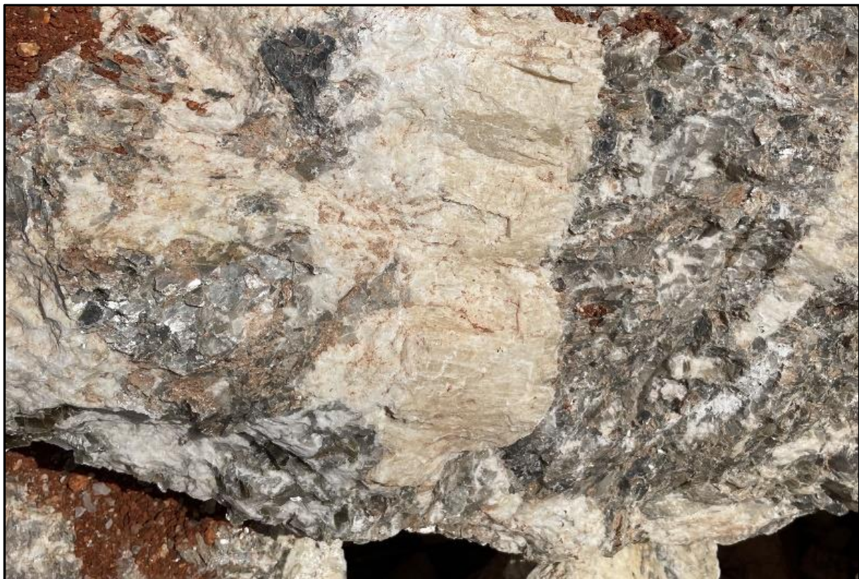
Plate 1: Hand specimen showing flake mica (grey), with potassium feldspar (cream), albite (white) and quartz (grey)
