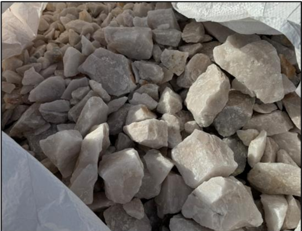
Plate 3: Crushed and screened quartz in bulk bag, selected from historical waste dump
