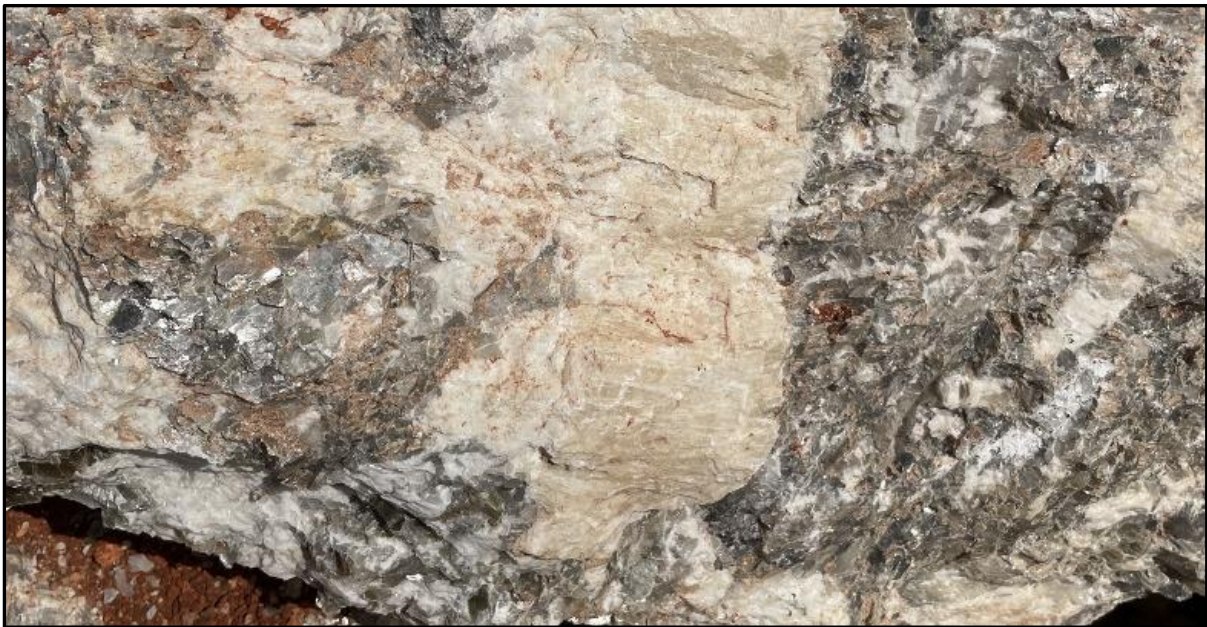
Plate 1: Hand specimen showing flake mica (grey), with potassium feldspar (cream), albite (white) and quartz (grey)
