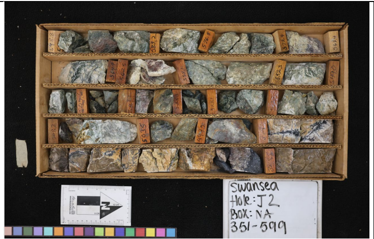
Figure 6: Drill core (split for sampling) from Swansea.
