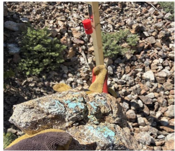
Figure 10: Secondary copper mineralisation (chrysocolla) within altered granite at TUC. Monument peg for claims held by Infinity shown in background.
