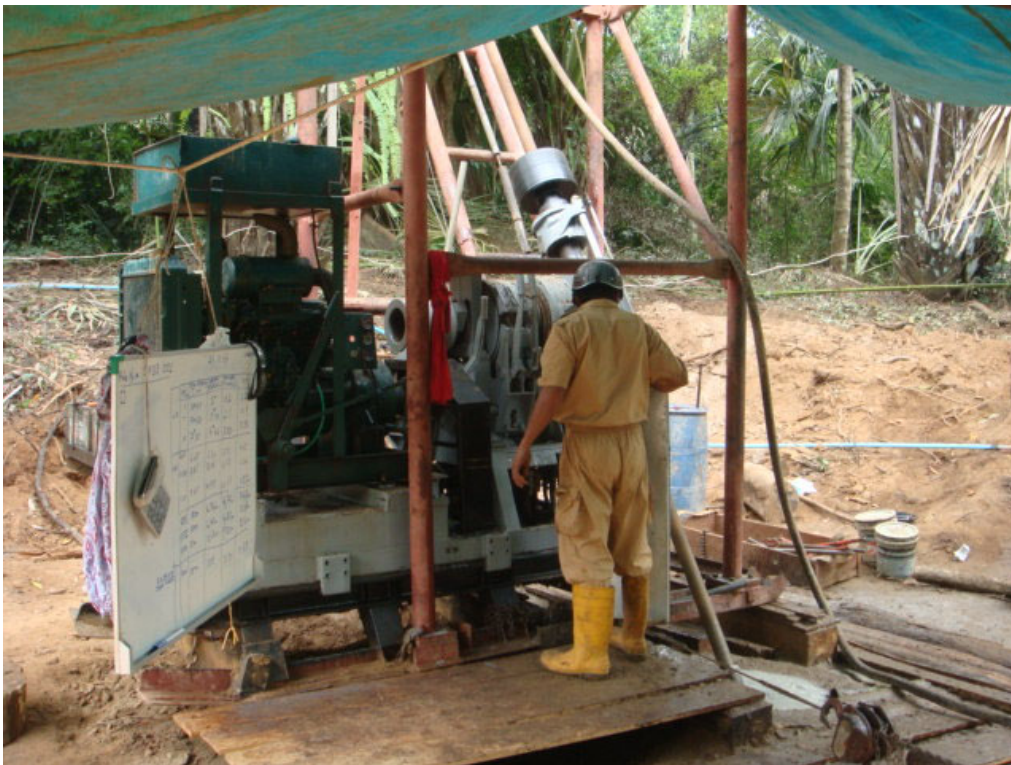
Figure 1. Diamond core drilling at Snoul Gold Prospect, Snoul MOU, north-eastern Cambodia.
