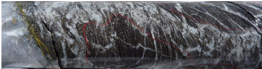
Figure 2. Small scale brittle-ductile deformation of albite-biotite-carbonate breccia vein (BSRCD201, 146.65m; 32ppm Au) producing parasitic fold hinge.
