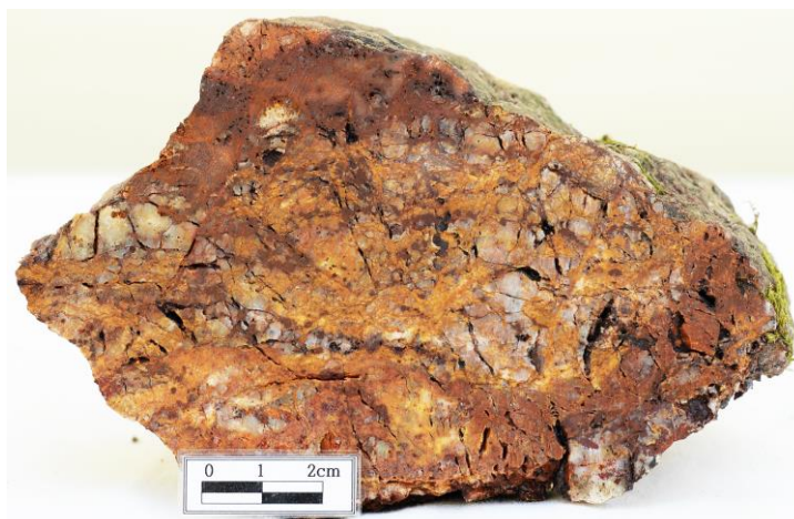
Photo 12. KRS200092: 27.8g/t Au, 29.4g/t Ag, 0.21% Pb, 0.03% Zn Sheared quartz vein with significant hematite (with peak Au result).
