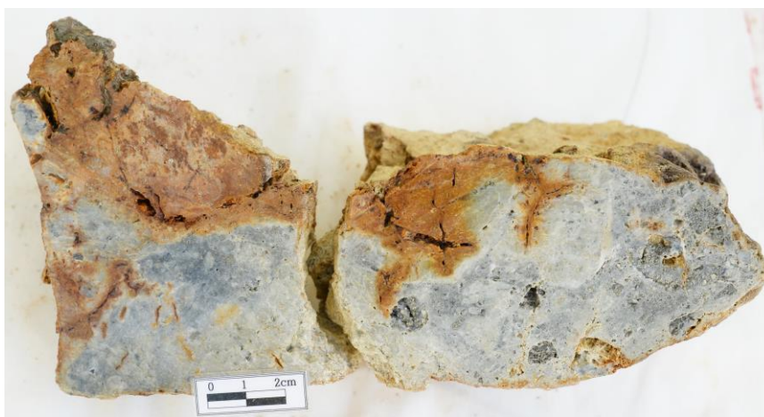
Photo 12. KRS200092: 27.8g/t Au, 29.4g/t Ag, 0.21% Pb, 0.03% Zn Sheared quartz vein with significant hematite (with peak Au result).
