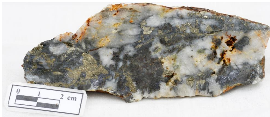
Photo 11. KRS200090: 16.8g/t Au, 170g/t Ag, 0.94% Pb, 0.34% Zn Hydrothermal breccia with significant silica-sulphide matrix and vuggy silica development.
