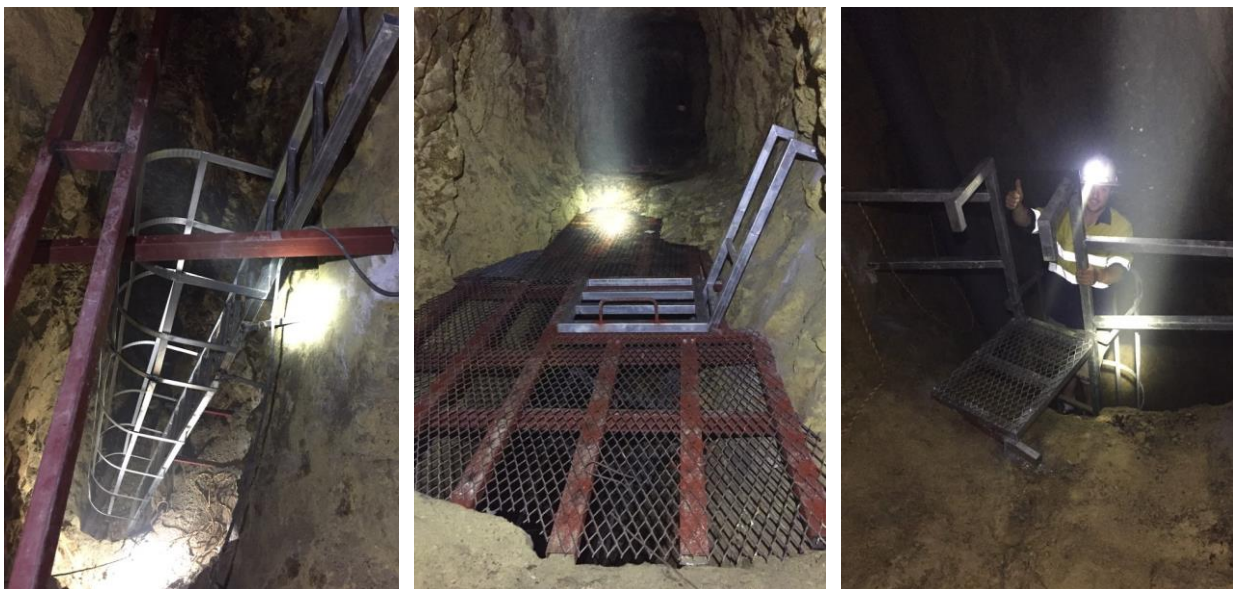
Photos 5, 6 and 7: Weolyu sublevel platform and access with Top level ladder way access at 325mRL.
