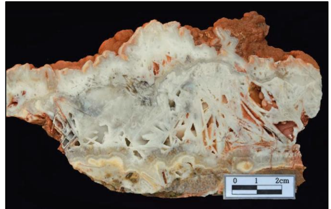
Photo 4: KRS203114. Results below detection limits. Multi-phase vein sample comprised of rhythmically banded chalcedonic silica with a core of chalcedonic quartz cemented quartz pseudomorphs after bladed calcite. Central Beopseongpo Vein Segment.
