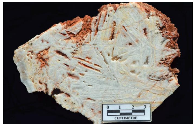
Photo 6: KRS203043. Precious metals below detection limits. Vein sample comprised solely of quartz pseudomorphs after bladed calcite, indicative of flash boiling. Central Beopseongpo Vein Segment.
