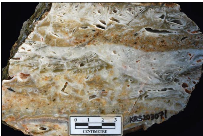
Photo 5: KRS203071. Precious metals below detection limits. Multiphase hydraulic vein breccia with quartz pseudomorphs after bladed calcite. Central Beopseongpo Vein Segment.
