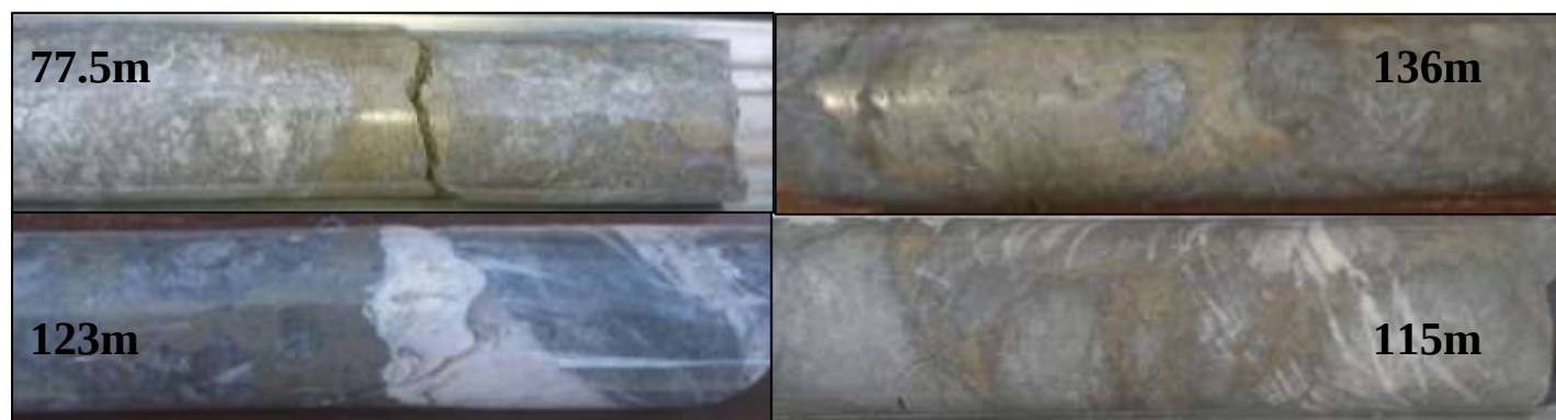
Figure 9. Examples of pyrite-arsenopyrite vein styles and orientations from Hole CMIPT64 from down hole depths shown. Similar veins are seen in Holes 65 and 66. All contain silver .
