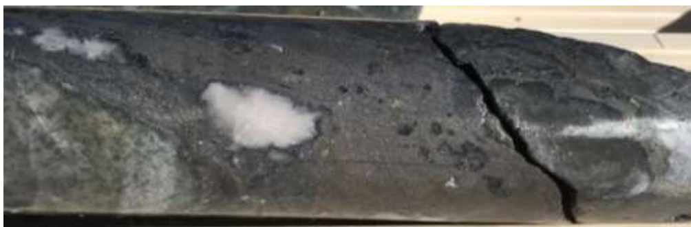
Figure 4. High grade “feeder vein” at 114.5 metres depth in Hole 63 containing silver, zinc, lead and copper with accessory molybdenum, antimony, tin and bismuth.
