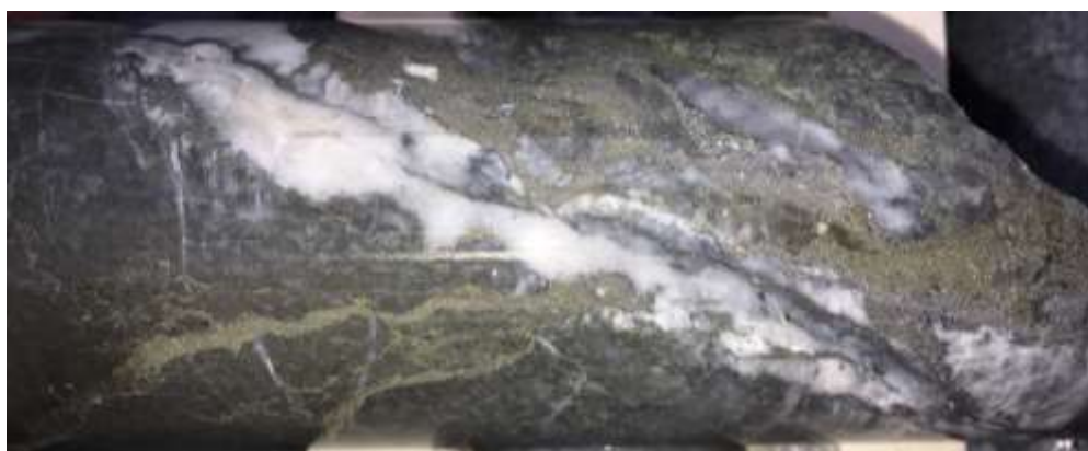
Figure 5. Quartz-pyrite-arsenopyrite-silver vein and stockwork from 77 m depth in Hole 63.
