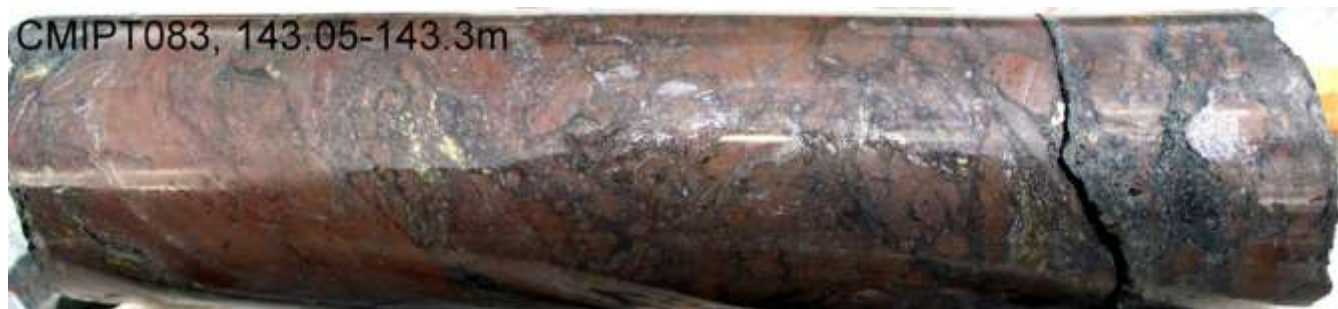
Figure 10. Hole CMIPT083: massive and brecciated massive sphalerite (red-brown) with lesser galena. Up to 3% chalcopyrite (yellow) is present in places.
