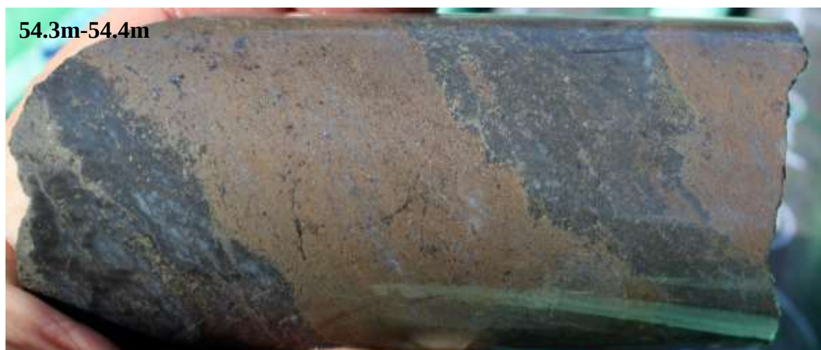
Figure 9. Hole CMIPT084: Photographs of end-member styles of massive sulphide mineralisation: massive pyrite (bronze colour) with fine grained sphalerite and galena (upper) and massive sphalerite (red-brown) with galena (silver grey) (lower). Similar styles of mineralisation occur in all four drill holes at Main Shaft.
