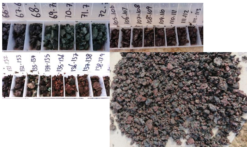
Figure 8. Alteration in Hole APIPT001. Strong chlorite-epidote alteration (top left) passes into strong hematite alteration (top right) then strong K-feldspar alteration in a porphyritic unit (bottom left). A close up of the strong K-feldspar unit is shown in the bottom right from 137 metres downhole and is typical of more proximal alteration.
