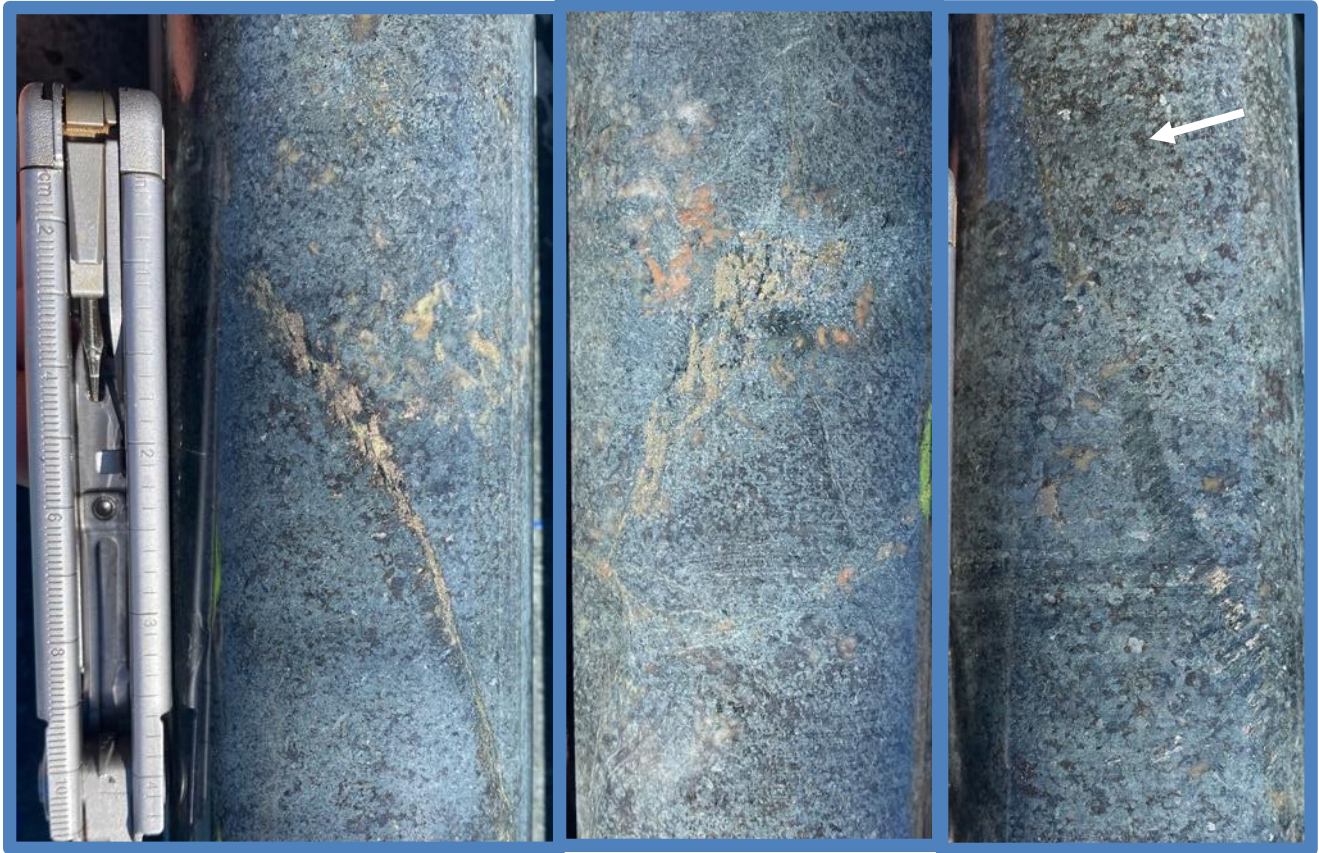
Figure 5. Photographs of diamond core from selected intervals from 95 metres to 98 metres down hole in RWIPT016. The photographs show disseminated to blebby to vein hosted sulphide mineralisation comprising pyrite-pyrrhotite-chalcopyrite (copper sulphide) and lesser pentlandite (nickel sulphide). Fine grained disseminated sulphide occurs in many places in this interval (see arrow for example).
