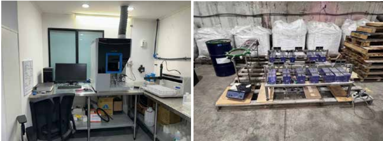
Figure 1.12. (L). ICP analytical machine capable of reading up to 66 elements to ppb levels of detection.
