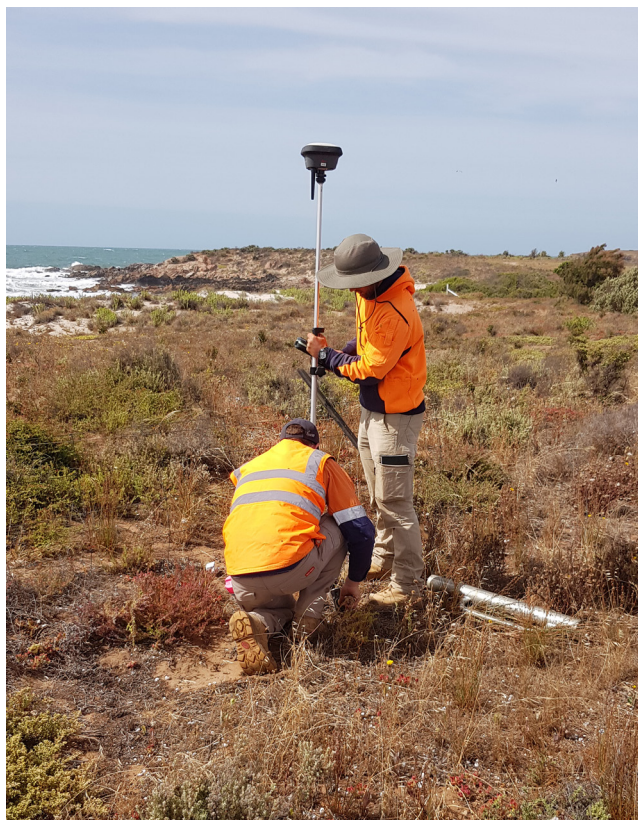
Surveying of control point at Cape Hardy
