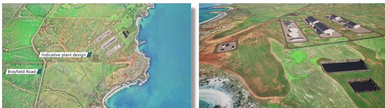
Rendered image of proposed 260ML/day desalination plant reference design at Cape Hardy (source- Northern Water).
