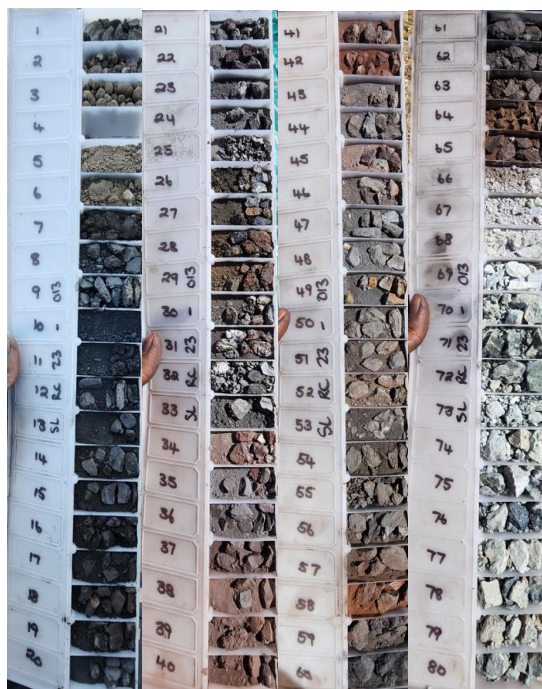
Figure 3. Chip tray photographs from hole SLRC23-013. The image shows a 60m interval of graphite mineralisation from 6m to 66m downhole. True thickness is unknown.
