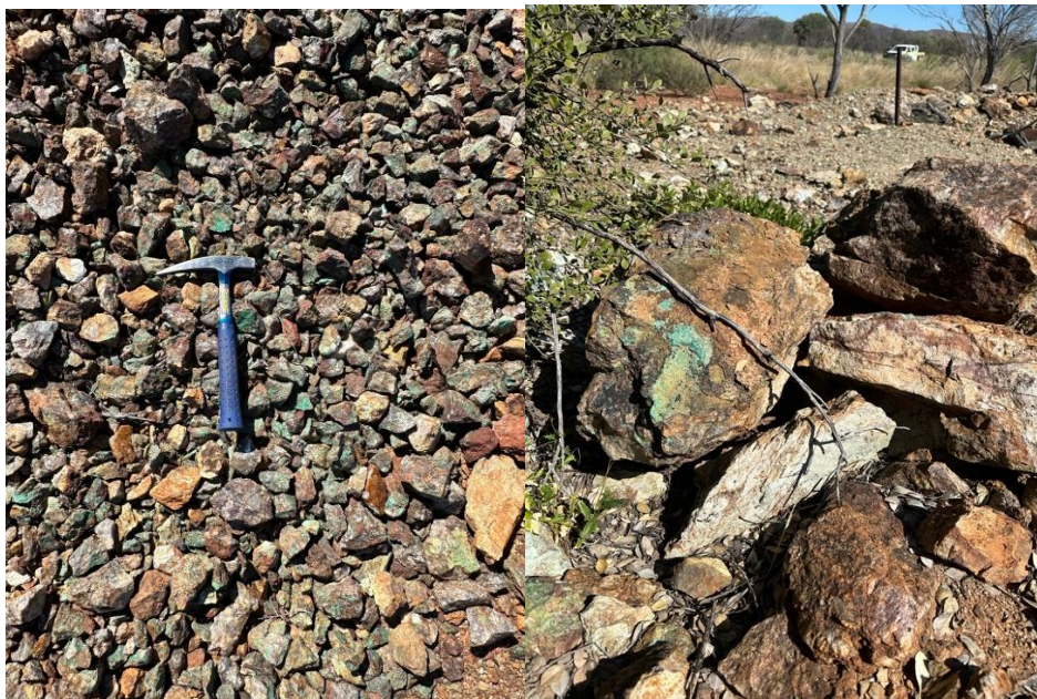
Figure 6. Examples of copper mineralisation at the Reward copper mine, containing green malachite and chrysocolla(copper)mineralisation.
