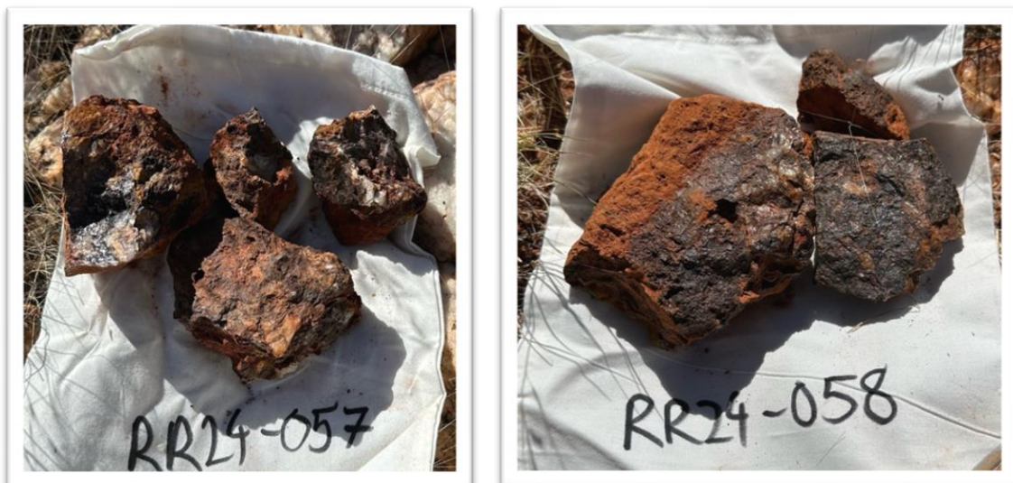
Figure 5. Rock chip samples of gossanous quartz veins from over the EM anomaly at the Scimitar Copper-Gold prospect. RR24-057 assayed 1.05g/t Au and 0.25% Cu and RR24-058 assayed 0.3g/t Au and 0.18% Cu.
