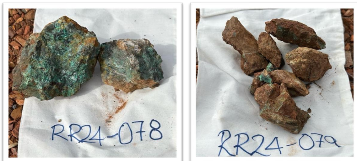
Figure 2. Rock chips taken for copper mineralisation at the Stanley Copper Prospect. RR24-078 assayed 29.1% Cu, 0.83g/t Au and 27.4g/t Ag and RR24-079 assayed 10.3% Cu and 0.2g/t A.
