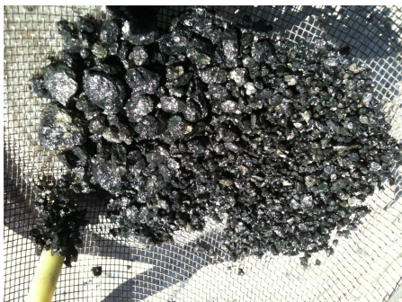
Photograph above of the high grade magnetite skarn zone in 12JRRC004, 67-68m showing visible pyrite and chalcopyrite
