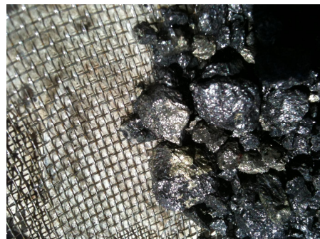
Photograph above of the high grade magnetite skarn zone in 12JRRC004, 67-68m showing visible pyrite and chalcopyrite
