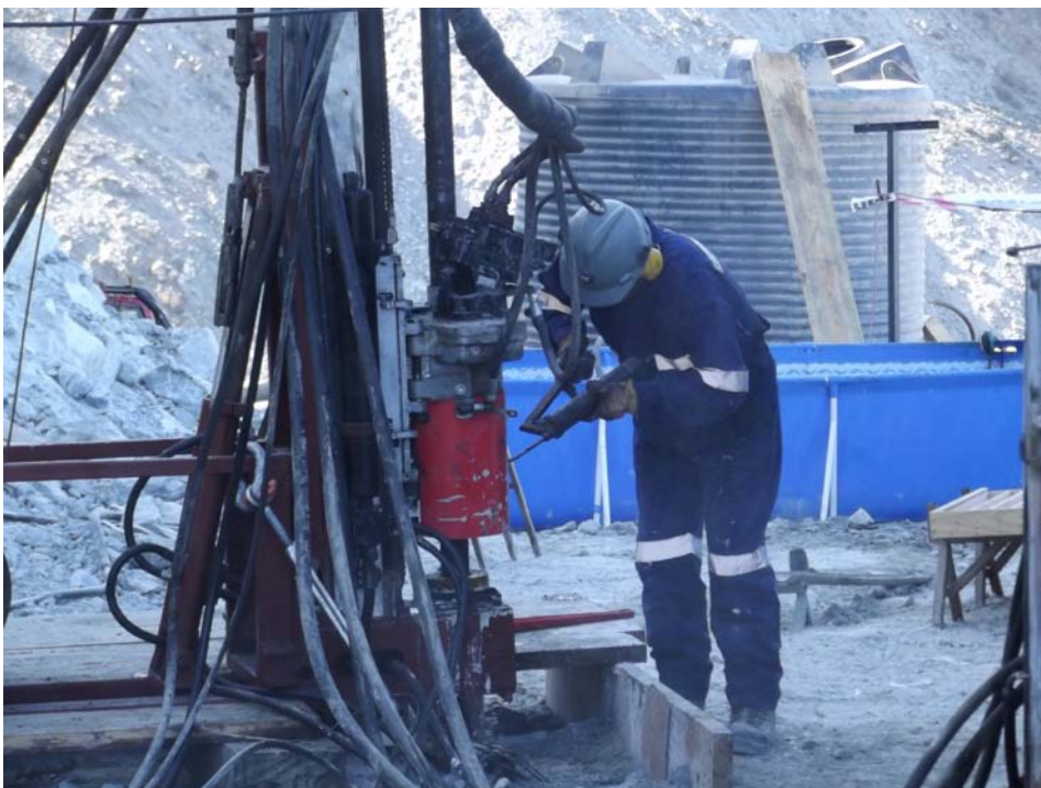
Current drilling on Platform B on which three diamond drill holes will be drilled to test a section of the target Cu-Au mineralised breccia.
