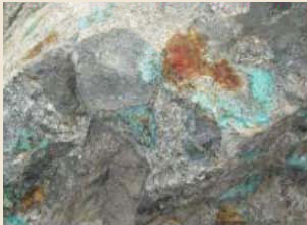
Figure 7. Breccia mineralisation, Cu sulphide nucleus, borders of Cu oxide, limonite in matrix
