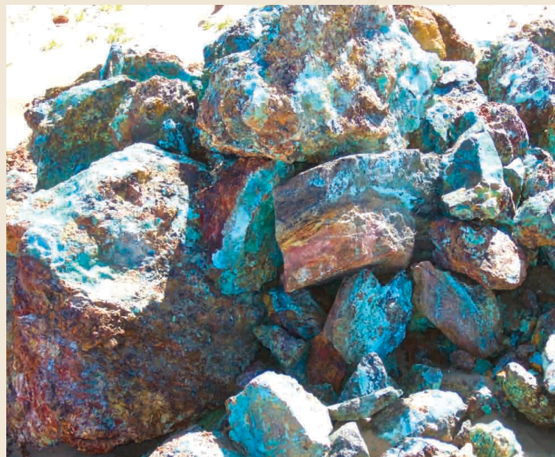
Breccia mineralisation, Cu sulphide nucleus, borders of Cu oxide, limonite in matrix
