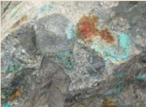
Breccia mineralisation, Cu sulphide nucleus, borders of Cu oxide, limonite in matrix
