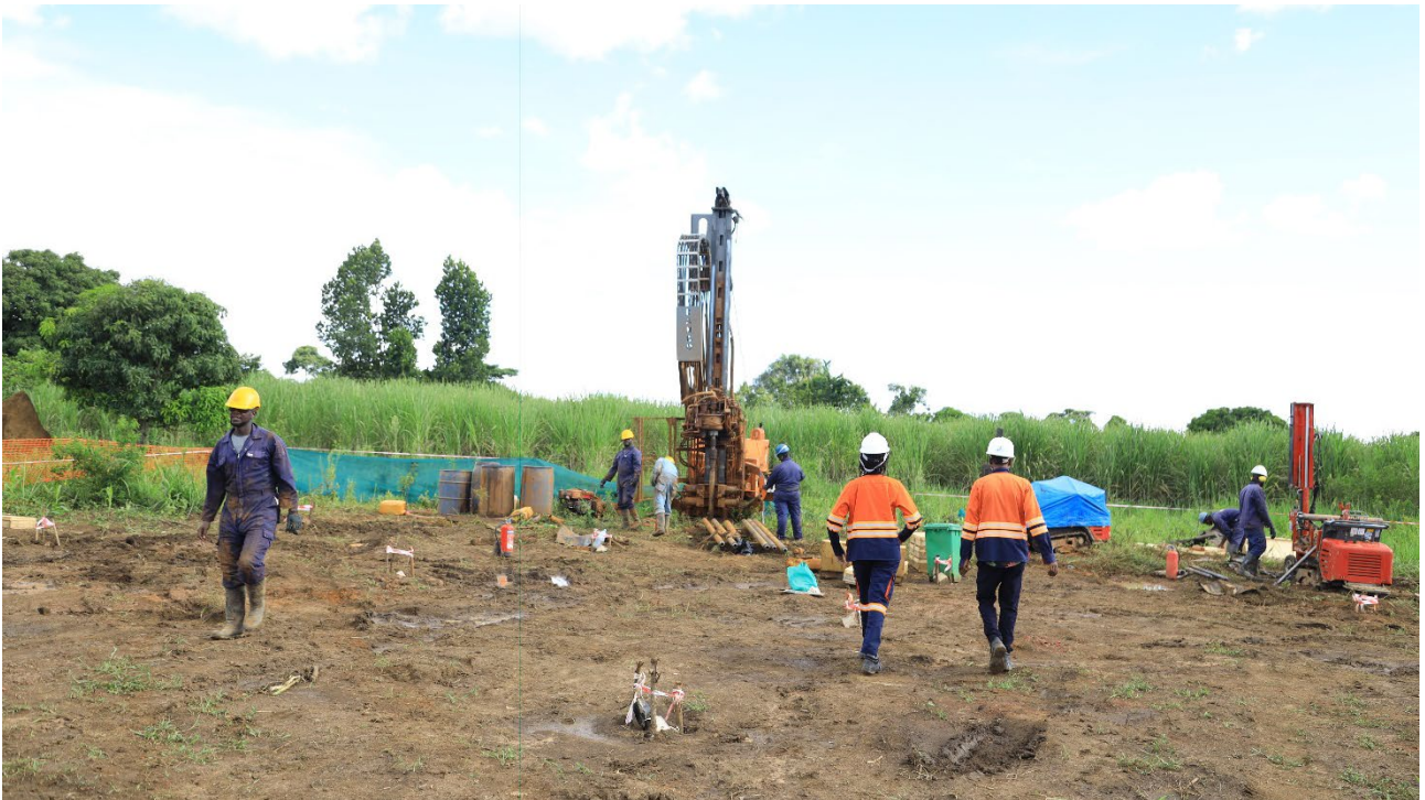
Figure 9: Makuutu Demonstration Plant test pit grade control drilling at test pit site No1 on 5m x 5m grid.
