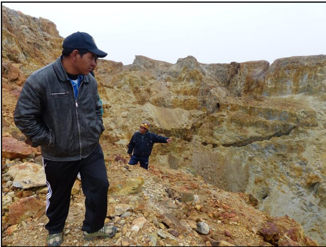
Figure 3 – A Large Glory Hole in the Porphyry at the Top of the Siglo XX Mine, with Members of the Juan del Valle Mining Cooperative
