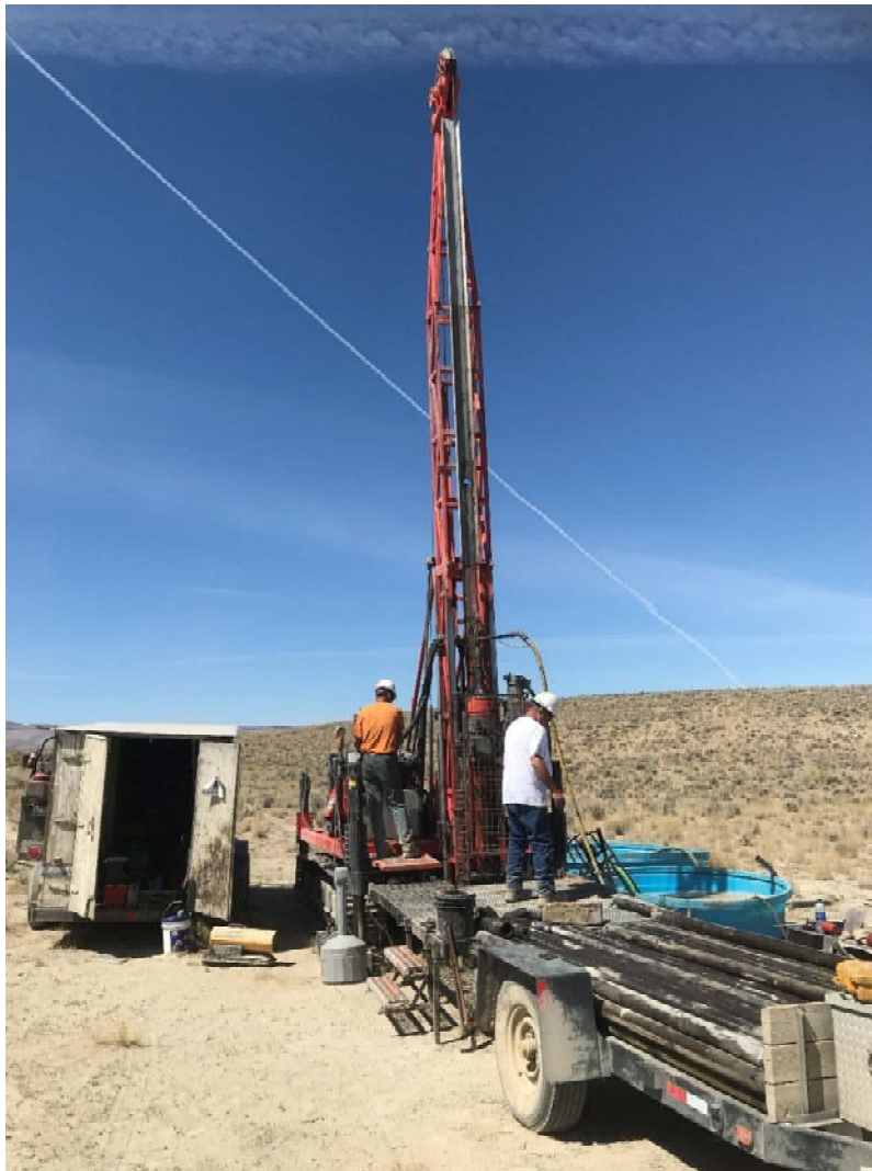
Figure 3 – Core drilling at McDermitt
