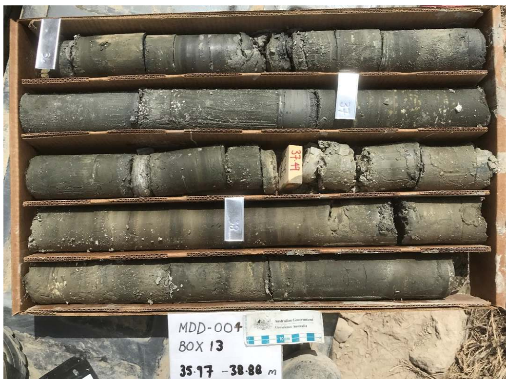
Figure 4 – Drill core from hole MDD-004 at McDermitt showing excellent core recovery through a lithium mineralised zone.
