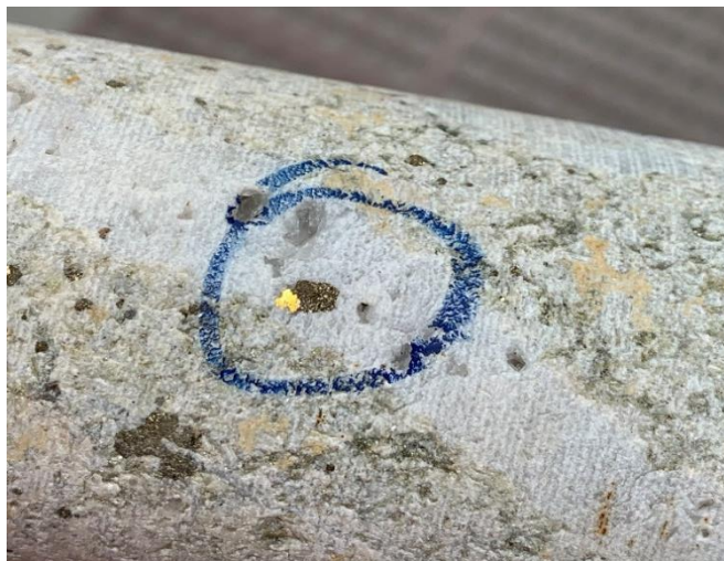
Figure 1 and 2: Underground drill core being inspected and drill core showing routinely logged visible gold which is generally a good indicator of high-grade mineralisation.
