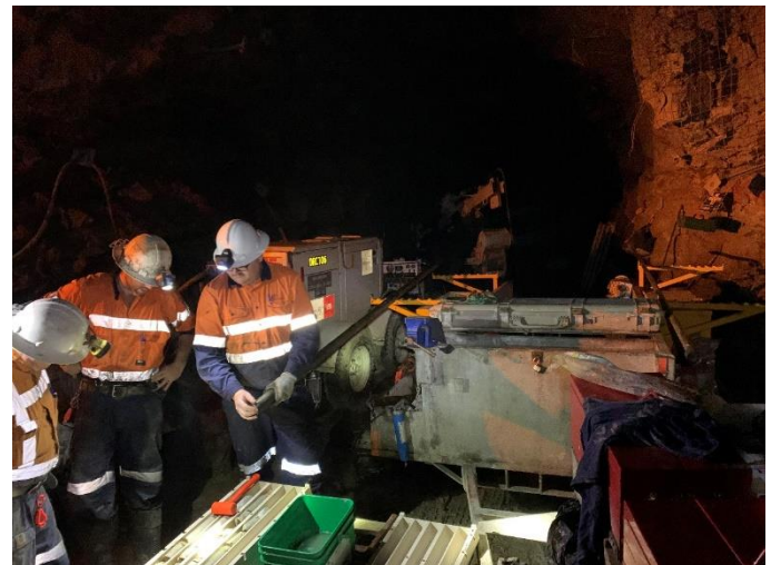
Figure 1 and 2: Underground drill core being inspected and drill core showing routinely logged visible gold which is generally a good indicator of high-grade mineralisation.
