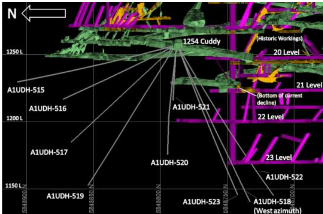
Figure 9: Long section looking east showing drilling traces, modern drives and stopes (green) and the interpreted historic workings (magenta and yellow).
