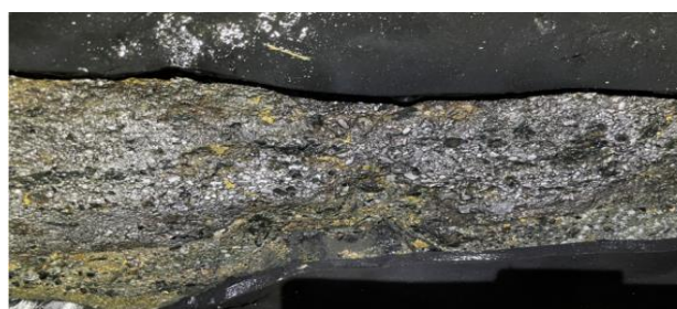
Figure 2 : Mill liner replacement works and visible gold embedded in liners prior to removal
