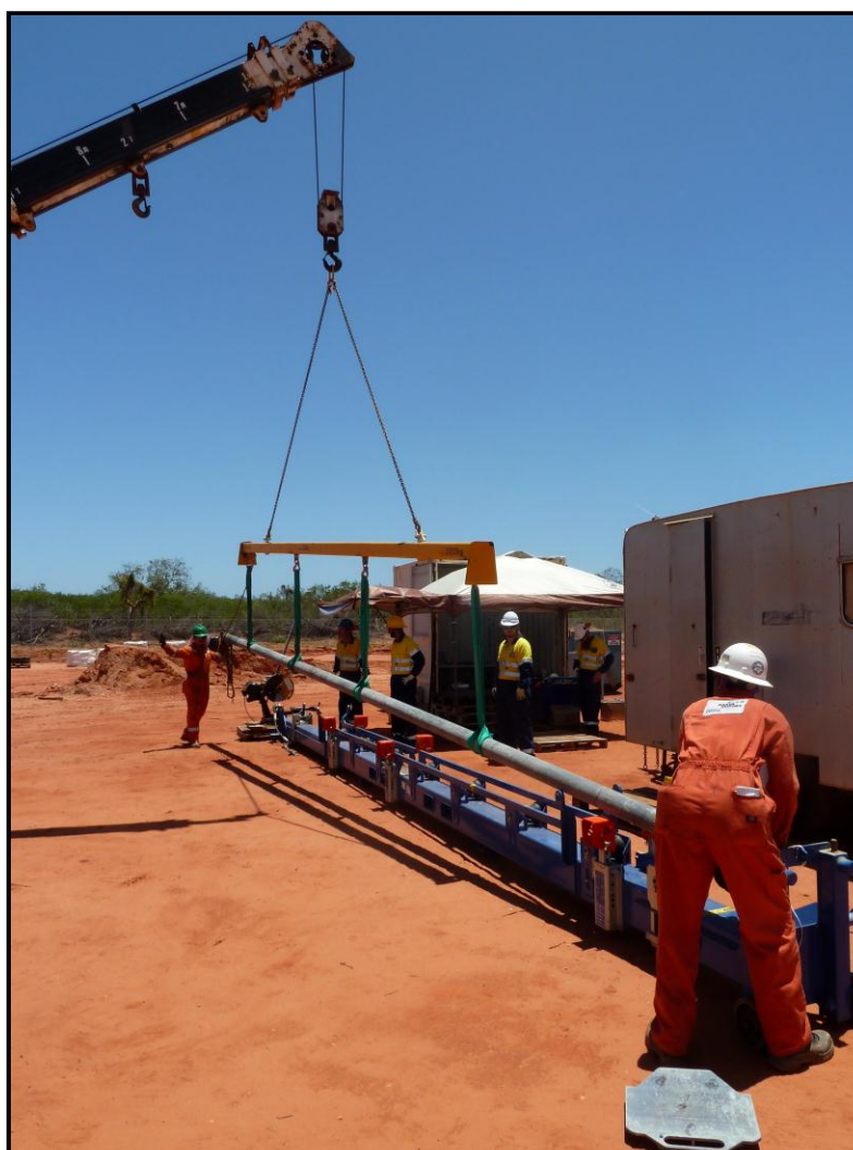
Lowering the core from the Goldwyer Formation into position for cutting, analysis and logging.
