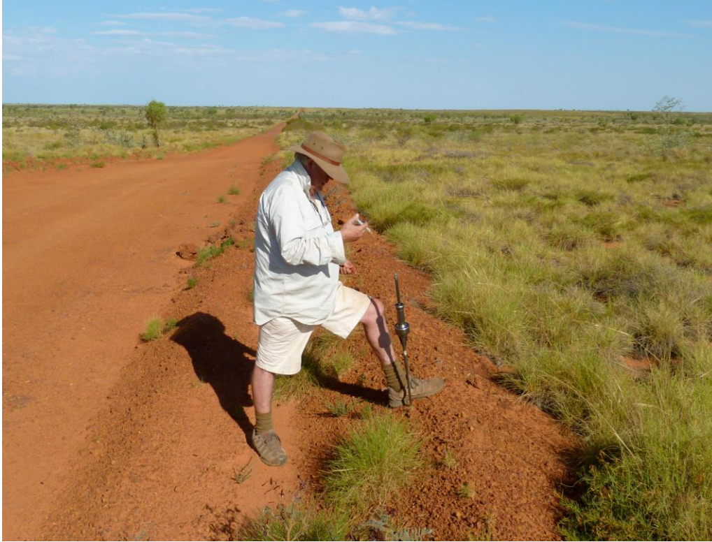
Geochemical personnel taking a hydrocarbon sample from the soil using a probe and syringe
