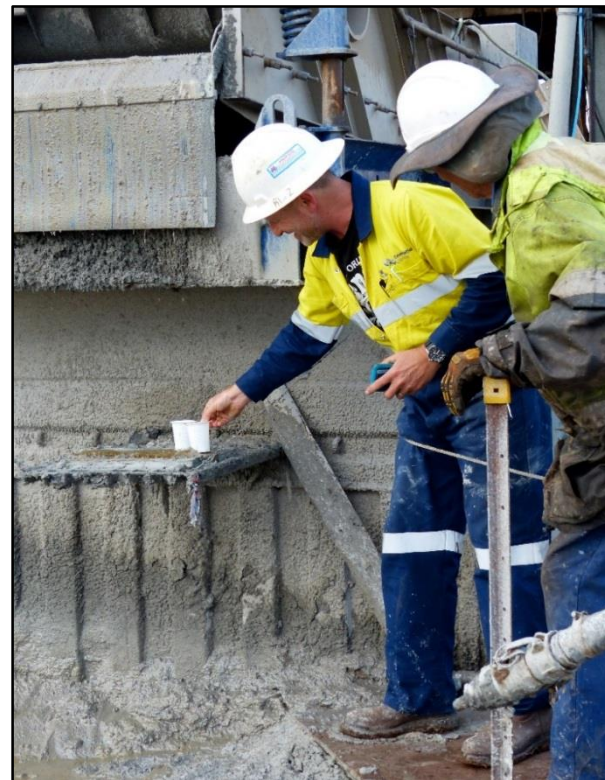
Wellsite Geologist Len Diekman collecting live oil samples from the shale shakers during drilling operations
