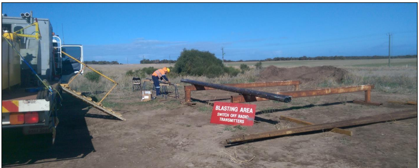
Preparation of perforating guns (above left), inserting guns and detonators into gun carriers (above right) and Westlog wireline unit and gun carriers (x2) and safety joint on racks (bottom)
