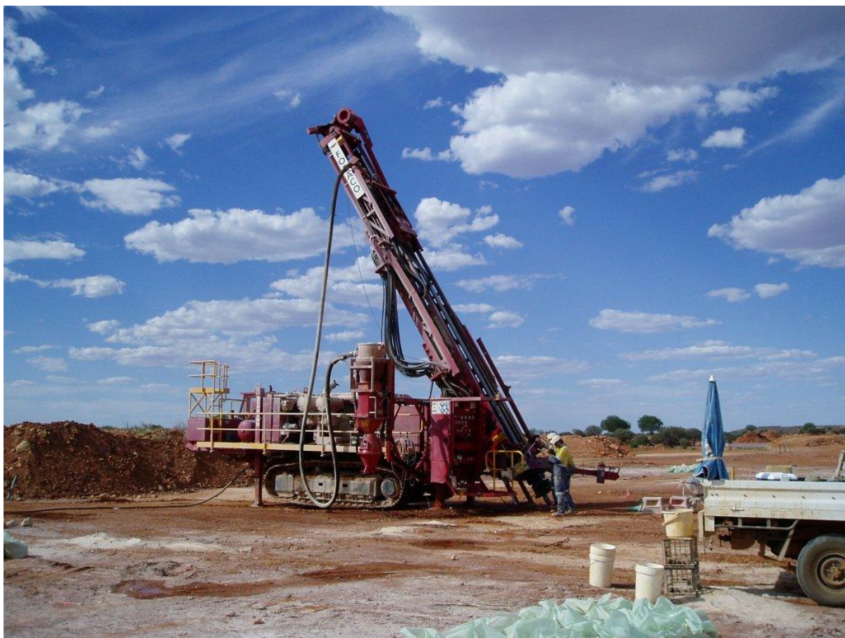
Figure 1 Air-core drilling adjacent to Reward Pit, Burnakura
