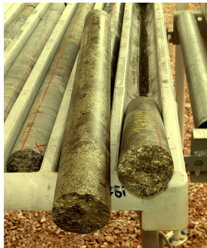
Chalcopyrite in drill core from Hole RJ 205 508m – 509m down hole
