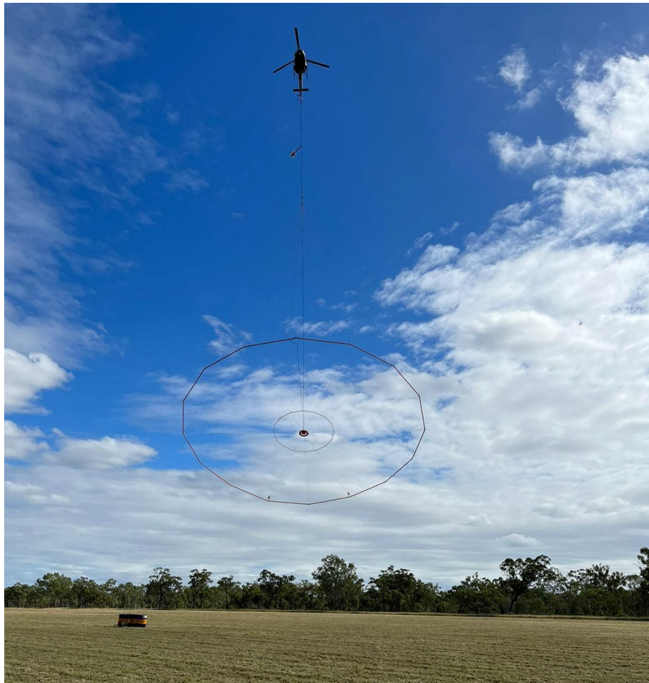
Figure 1. Airborne VTEM Survey at Ravenswood North.
